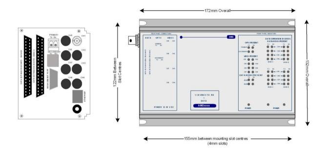
The **AMG3717E-DR-SF** is a standalone single channel video insert unit designed to transmit 1 video signal and transmit and receive up to 16 data or audio signals together with Ethernet over one singlemode fibres with Dual Redundant ring. The 16 data/audio channel interfaces, whether RS-232, RS-422, RS-485, 20mA, TTL, Contact Closure, Lonworks or Audio, are defined at manufacture by the addition of daughter boards fitted onto the Data Expansion Board A & B.
