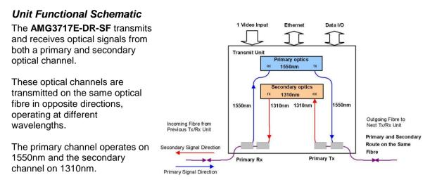
The AMG3717E-DR-SF receives and drops off data and Ethernet signals transmitted from an AMG3788EN-DR-SF receiver. It then inserts video, data and Ethernet signals onto the outgoing optical signal.
